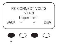
When the Upper Limit is displayed, the desired compensated voltage has been stored and the < - > and < + > soft keys can be released.
