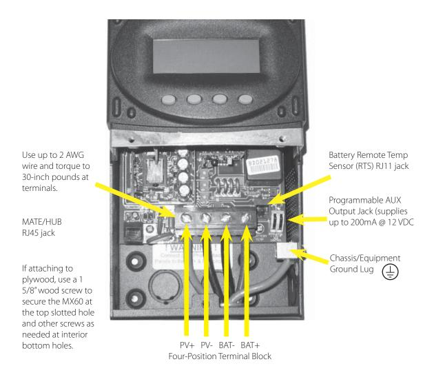
The PV (-) and BAT (-) terminals are connected internally. Only one negative wire may be needed to connect to the Four-Position Terminal Block if the PV - and BAT- conductors are bonded at the negative bus bar. See Figures 2 and 3 for sample wiring diagrams.
