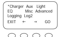
Press  $\leftarrow$  or  $\rightarrow$  to move the asterisk "\*" to the left of the desired screen. The asterisk allows access to any screen to its right.
