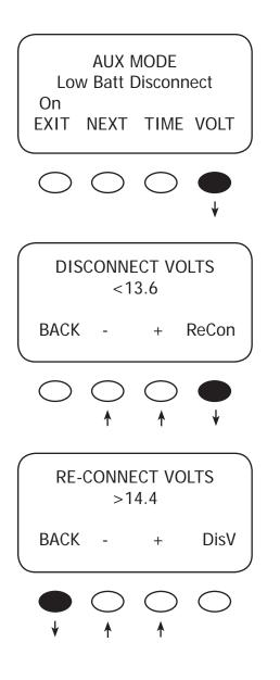
In the Low Batt Disconnect screen, press the **<VOLT>** soft key to adjust the battery voltage disconnects set point.
