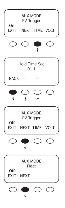
To adjust the minimum amount of time the PV voltage must remain high before deactivating the AUX MODE, press the **<TIME>** soft key.
