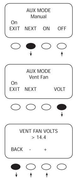
Press the **<ON>** or **<OFF>** soft keys to manually activate or deactivate AUX MODE. Press the **<NEXT>** soft key to view the Vent Fan screen. To view other screens, continue to press the **<NEXT>** soft key.
