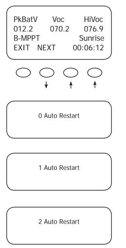
Pressing and holding the #4 soft key for several seconds selects among the three MX60 Auto ReStart modes: 0, 1, and 2 (default). Auto ReStart allows the MX60 to perform internal recalibrations and eliminate any possibility of software errors. To change the mode, release the #4 soft key and press and hold again.
