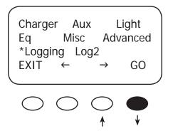
From the MAIN Menu, press the  $\langle \rightarrow \rangle$  soft key to move the asterisk next to the *Log2* function and then press the  $\langle GO \rangle$  soft key.
