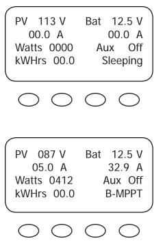
Turn the PV input breaker on. The MX60 automatically detects the PV input voltage. (Note: If PV voltage registers "000V" when the breaker is on, please check the polarity of the PV wires.)
