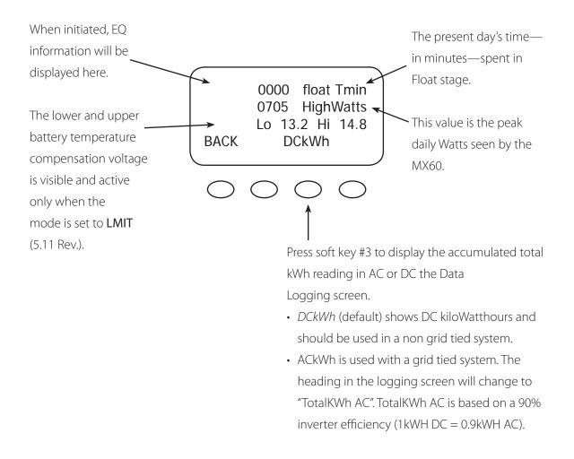
**Note:** Float time does not accumulate (1) when the MX60 is sleeping or (2) when an external power source keeps the battery above float voltage.
