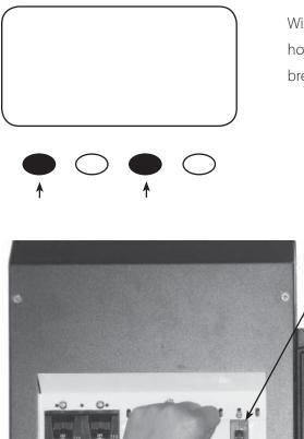
With the PV array and battery breakers off, press and hold soft keys #1 and #3 and then turn on the battery breaker (see Figure 4).
