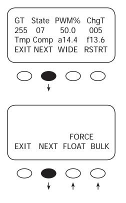
From the MISC screen, press the **<NEXT**> soft key to view the FORCE, FLOAT, or BULK screen.
