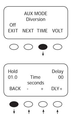
Press the **<TIME**> soft key to advance to the Time screen which allows the user to adjust the minimum time the AUX MODE is active after the battery voltage falls below the Hysteresis voltage.
