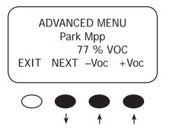
Press the <-VOC> or <+VOC> soft key to select one of the 13 fixed percentage values. Park Mpp applies to Auto Sweep Mode if the output current is less than 5 amps; U-Pick always uses the Park Mpp value. Press the <**NEXT**> soft key until the MPPT Mode screen appears.
