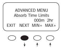
In the Absorb Time Limits screen, the user can set the minimum and maximum times the MX60 stays in the Absorb recharge cycle.
