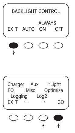
AUTO (default) leaves backlight and soft keys on for 60 seconds whenever any soft key is pressed (pressing any soft key when the LCD is *not* lighted does not change any settings).
