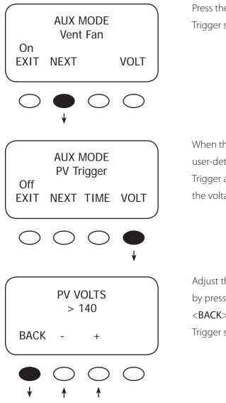
Press the <**NEXT**> soft key to advance to the PV Trigger soft screen.
