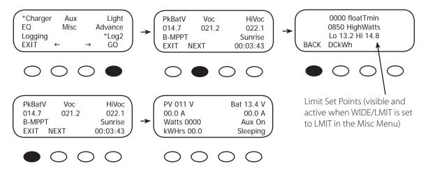
After confirming the Upper Limit and Lower Limit voltages, press the <←> soft key in the MAIN Menu. Press the <**GO**> soft key to advance to the first MISC screen. From this screen, you can access MISCELLANEOUS Screen 2.
