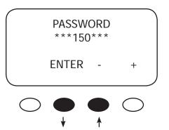
Press the " – " soft key until the password 141 shows on the screen. Press the **<ENTER>** soft key to return to the BATTERY VOLTAGE.
