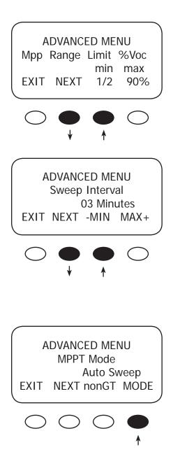
In the ADVANCED MENU screen, press the **<NEXT**> soft key until the Mpp Range Limit % VOC screen appears. Press the **<1/2**> soft key until FULL appears. When finished, press the **<NEXT**> soft key to go to the Sweep Interval screen.
