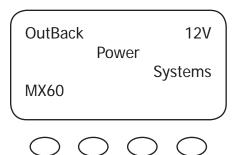
The MX60 briefly returns to the Power-Up screen and then automatically opens the STATUS screen which displays information regarding the recharging status. Confirm the battery voltage displayed in the upper right corner is correct.
