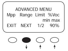
Use ½ value for high input arrays to speed up initial sweep.
