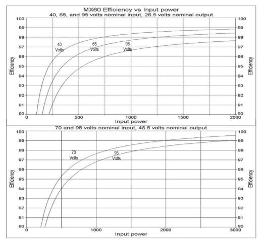
Figure 6 24V and 48V Battery System Efficiency Curve
