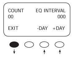
Use the <-DAY> and <+DAY> soft keys to preset the interval day to initiate an automatic equalization cycle. The EQ INTERVAL displays the number of days in the interval between cycles and COUNT displays how many days of the interval have passed.
