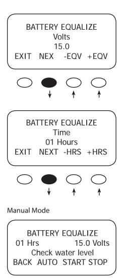
Press either the < -EQV> or <+EQV > soft key to change the EQ voltage, following your battery manufacturer's recommendations. Note that the factory default EQ voltage is set low, the same as the factory default Absorb voltage. Press the <NEXT> soft key to view the BATTERY EQUALIZE Time screen.
