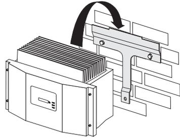
4. Use the provided M6x12 screws to fix the inverter and prevent it from being lifted out of place.
