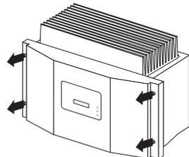
5. Remove the protective conductor (PE) connection from the lid by loosening the locking device of the PE connection on the lid.
