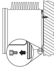
5. Remove the inverter upwards from the wall mounting bracket.
