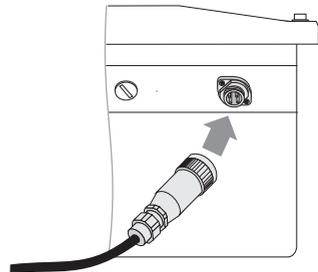
The AC cable is now connected to the inverter.
