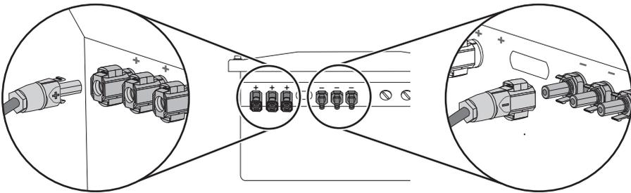
4. Close all the DC inputs that are not needed as described in section 5.4.4 "Connecting the Small Wind Turbine System (DC)" (page 29) in order to create the sealing on the inverter.
