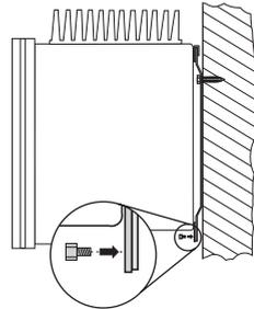
5. Check to ensure the inverter is firmly fastened.
