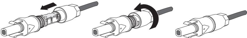
☑ The DC plug connectors are now assembled and can be connected to the inverter as described in section 5.4.4 "Connecting the Small Wind Turbine System (DC)" (page 29).
