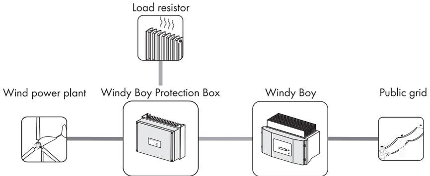
Furthermore, the Windy Boy can be used as an inverter for power conversion units based on the permanent magnet generators (hydro power systems, combined heat and power plants, diesel generator, etc.). The manufacturer of the small wind turbine system or the generators should have his system set up for operation with the Windy Boy (see also the Windy Boy planning guidelines in the download area at [www.SMA.de/en](http://www.SMA.de/en)).
