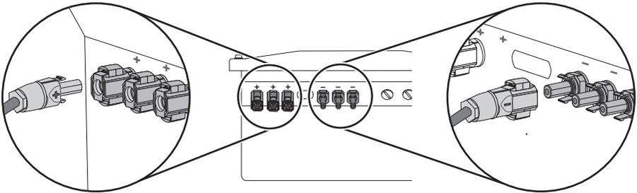
2. To create the sealing on the inverter, all the DC inputs that are not needed have to be closed as follows:
