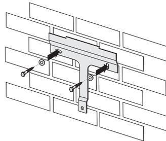
3. Use the upper mounting clips to fit the inverter in the wall mounting bracket so that it cannot be pushed out of the wall mounting bracket from the side.
