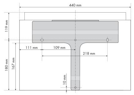
Figure 5: Wall mounting bracket dimensioning
