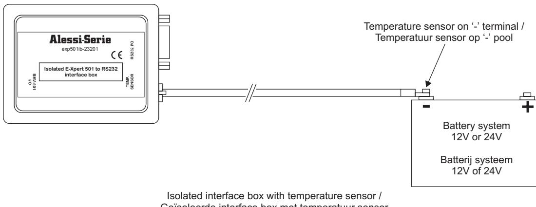
Note 1 : The temperature sensor cable sheath, is made of a 70°C flame retardant PVC compound according to VDE0472 part 804
