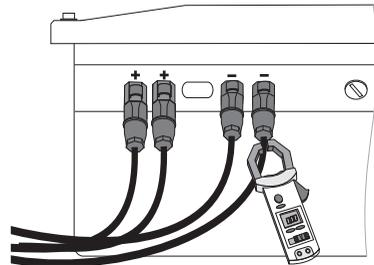
3. Unlock all DC connectors. For this purpose, use a screwdriver with a width of 3.5 mm.
