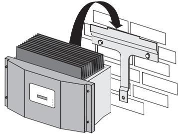
4. If a second protective conductor is required in the country of installation, ground the inverter and fix it securely, as described in section 5.2.3 "Connecting Additional Grounding" (page 25).
