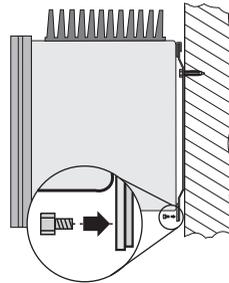
6. Check to ensure that the inverter is securely in place.
