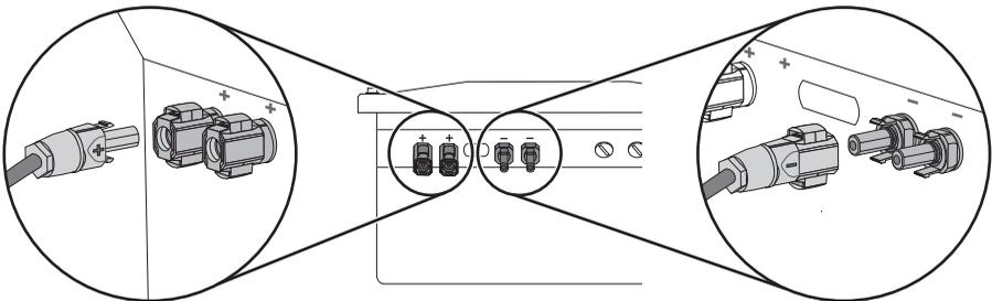
4. Close all the DC inputs that are not needed as described in section 5.4.4 "Connecting the Small Wind Turbine System (DC)" (page 31) in order to seal the inverter.
