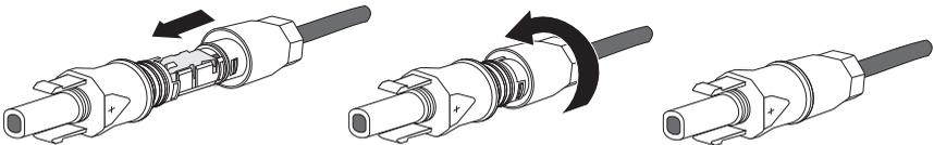
☑ The DC connectors are now assembled and can be connected to the inverters, as described in section 5.4.4 "Connecting the Small Wind Turbine System (DC)" (page 31).
