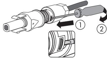
4. Declamp the clamping clip. For this purpose, use a screwdriver with a width of 3.5 mm.
