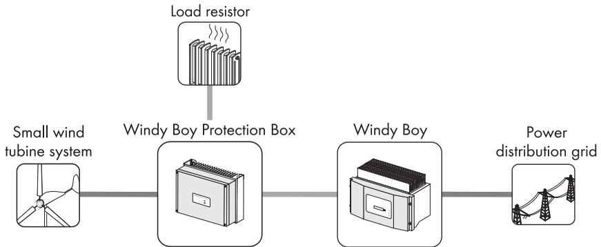
The Windy Boy can additionally be used as inverter for energy converters based on permanent magnet generators (hydro-power systems, combined heat and power plants, diesel generator, etc.). The manufacturer of the small wind turbine system or generator must have his plant approved for operation with this Windy Boy.
