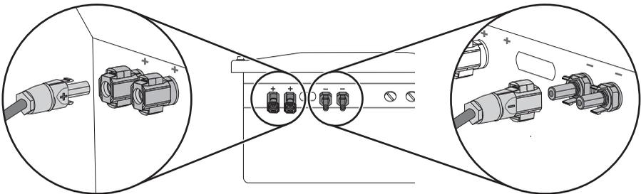
3. In order to seal the inverter, all the DC inputs that are not required have to be closed as follows:
