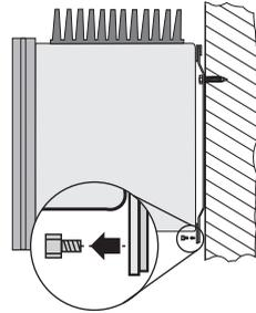
5. Lift the inverter off the wall mounting bracket.
