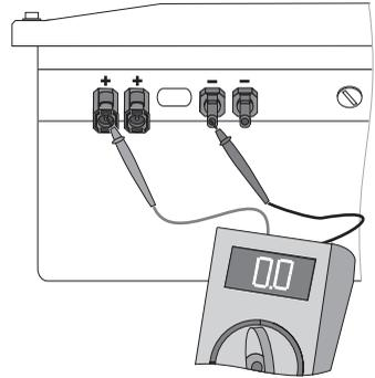
6. Measure the resistance between L1 of the small wind turbine and the ground potential.
