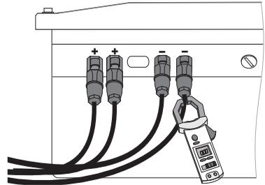
2. Unlock all DC connectors. For this purpose, use a screwdriver with a width of 3.5 mm.
