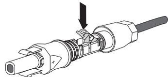
3. Ensure the cable is correctly in place:
