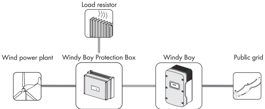
Furthermore, the Windy Boy can be used as an inverter for power conversion units based on permanent magnet generators (hydro power systems, combined heat and power plant, diesel generator, etc.). The manufacturer of the small wind turbine system or generator must have approved his plant for operation with this Windy Boy.
