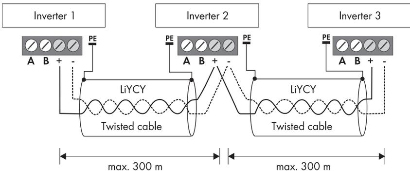
The length of the cables between 2 inverters must not exceed 300 m.
