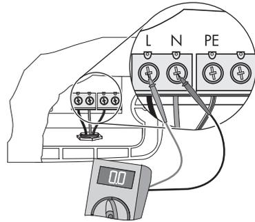
8. Verify the absence of voltage L to PE at the AC terminal with a suitable instrument.
