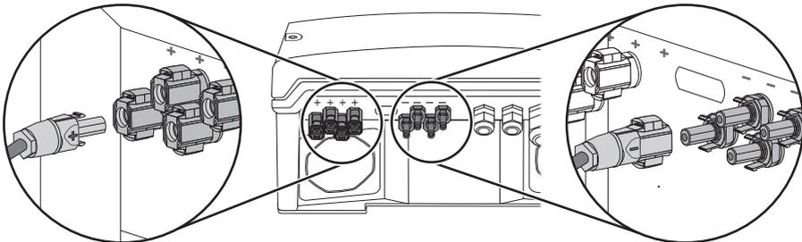
3. Close all unused DC inputs as described in Section 5.4.4 "Connecting the Small Wind Turbine System (DC)" (page 34) to seal the inverter.
