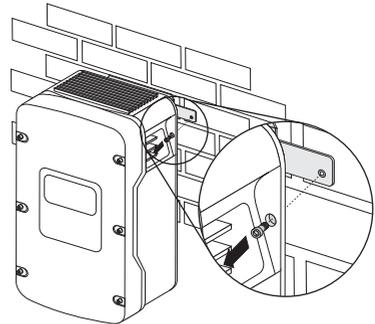
7. Remove the inverter from the wall mounting bracket by lifting it vertically upwards.
