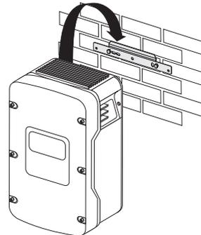
4. Screw the inverter onto the wall mounting bracket on both sides using the screws (M6x8) provided. Only fasten the screws hand-tight.
