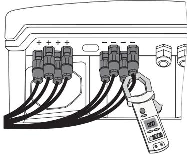
4. Release and pull off all DC connectors with a screwdriver (blade width: 3.5 mm):
