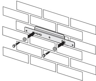
3. Attach the inverter to the wall mounting bracket using the special opening at the rear of the enclosure.
