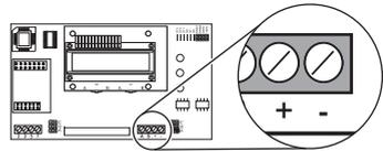
7. To connect the 3 inverters, connect the positive and negative cables from the 2 other inverters to the terminal block of the middle inverter.
