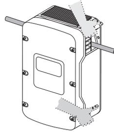
2. Secure the wall mounting bracket to the wall using appropriate screws and washers.
