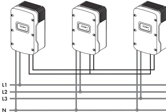
If this electronic circuit is activated, you can specify how the other two inverters should react if there is a device fault in the third inverter or a line voltage fault occurs in its phase.
