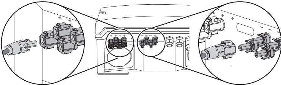
2. To seal the inverter, any unused DC inputs must be closed with DC connectors and sealing plugs.
