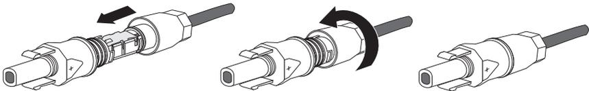
The DC connectors are assembled and can now be connected to the inverter as described in Section 5.4.4 "Connecting the Small Wind Turbine System (DC)" (page 34).
