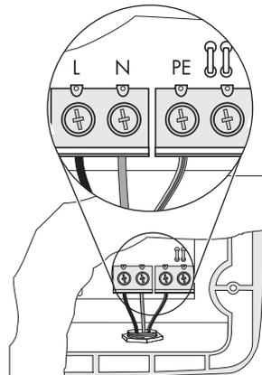
8. Fasten the cable gland tightly on the enclosure opening.
