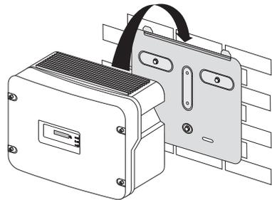
5. **Visual inspection:** The inverter is only correctly mounted when both rear panel mounting plates slightly protrude through the cutouts.
