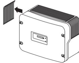
2. Clean the air grill with a soft brush, a paint brush, or pressurized air.
