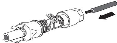
2. Press the clamping clip down until it audibly snaps into place.
