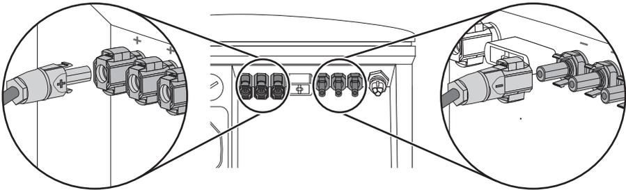
2. To create the seal on the inverter, all DC inputs that are not required must be closed as follows:
